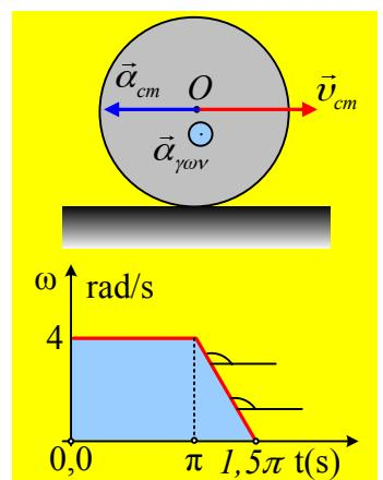
$$\alpha_{\gamma\omega} = \frac{dv}{dt} = \frac{\Delta v}{\Delta t} = \frac{0 - 4}{1,5\pi - \pi} rad/s^2 = -\frac{8}{\pi} rad/s^2$$
