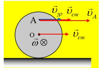
$$v_A = v_{cm} + v_{yp} = v_{cm} + \omega r = \omega R + \omega r = \omega(R + r) \rightarrow \\ v_A = 4(0,5 + 0,3)\text{m/s} = 3,2\text{m/s}$$
